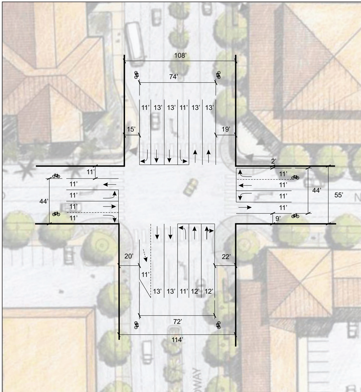
This figure combines the conceptual development plan reviewed by the community with projected intersection improvement requirements, including two northbound and two southbound lanes on Broadway and dedicated left-turn lanes on Napa and Leveroni Roads. The diagram also depicts desired design features, such as bike lanes, parking, cross-walks and planter strips.
